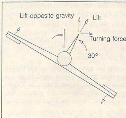
simulators, the pilot will increase the total lift by increasing the angle of attack. This keeps the 'lift opposite gravity' force constant so that no change in attitude will occur while turning.
