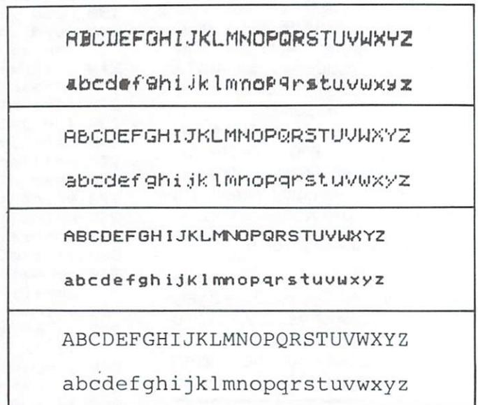
The alphabet on various CBM printers. From top to bottom: the MPS-801 (formerly the 1525); the MPS-801 with modified character set, available from Wilanta Arts of Mississauga; the MPS-802 (formerly the 1526); and (bottom) the DPS-1101 daisy wheel printer.
