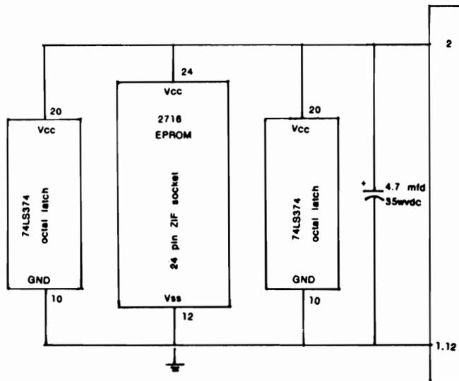
**Note:** As Vcc is 5 volts, the capacitor wvdc is not critical.
