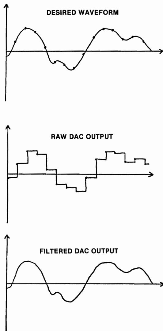
FIGURE 1: Operation of D-to-A Converter
