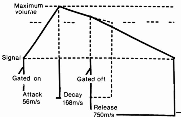
Here, it can be seen that the voice was gated off, i.e., released, before the envelope had decayed to its sustained level, but that, when the voice was released, it simply released from the point it had reached.
