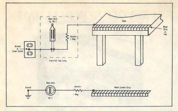
with a neon bulb and dropping resistor) to ground the metal strip. The resistor is necessary to prevent you getting a good zap of static charge; also a pulse isn't generated on the computer.  $\Box$
