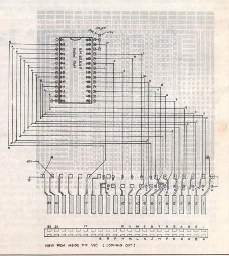
solder connections are very close together so care must be taken to prevent solder bridges. If there are any, the ohm meter will find them and they must be removed before you insert the chip and power-up. Extra time taken at this stage will prevent problems later on. Pads A, 1, and 22 on the edge connector should be shorted together, but make sure that there is no continuity between pads 21 and 22.
