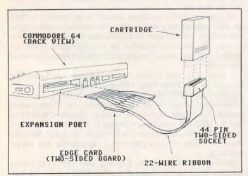
approximately 1/8 inch from the other end. I found it helpful to use an existing cartridge to make the measurement marks on the socket. I have heard that a ready-made 22 pin socket can be purchased for about twenty dollars (Cdn.), but I was unable to locate a vendor.
