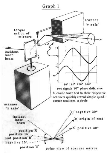
\*note . . . the projection angle is twice the deflection angle relative to the incoming beam or plane of light
