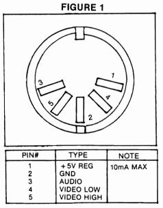
All we need be concerned with are pins two and three. Pin two is the ground. This is nothing more than a common point and, if your computer is hooked up right, will eventually wind up in the earth. It is used more or less as an electronic dump. Pin three is the audio signal. This is the
